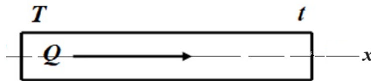
Figure 1 – Redistribution of thermal energy in the rod
